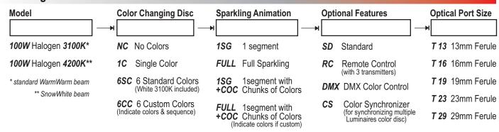
order e.g. for standard 100W Halogen 3100K c/w 5+1 color changing, 1 segment sparkling effect, standard feature & T16 port size ...100W-3100K-6SC-1SG-SD-T16
