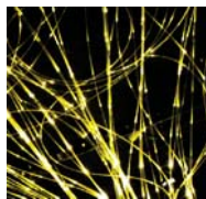
1.0mm diameter with clear jacket (O/D 2.2mm)
