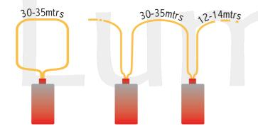
Note that for sidelight applications, 30 to 35 meters runs are ideal when looped back to a single luminaire. On long runs, multiple luminaires in series are the norm. Wherever possible, sidelight cable should always be looped in and out of the luminaire. They may or may not be synchronized depending on the color effect desired. When using multiple luminaire, cable run should be the same length as possible. This will ensure the cables uniform brightness.
