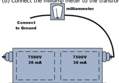
\*(c) Plug the input into a 120-volt receptacle or adjust Powerstat to read 120 volts on the voltmeter. Read the SHORT CIRCUIT M.A. on the milliamp meter and disconnect input plug.
